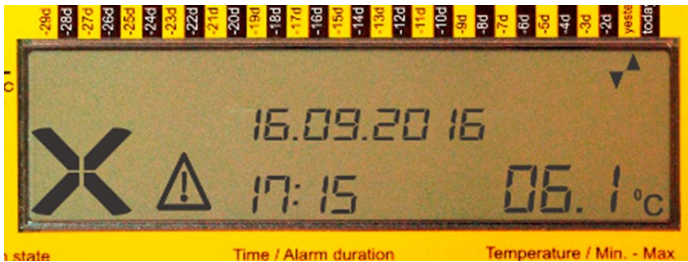
Figure 3 Current temperature reading with no preset alarm levels violation
