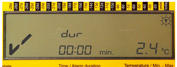
Figure 3 Current temperature reading with no preset alarm levels violation
