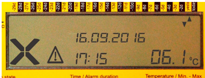
Figure 4 Current temperature reading with preset alarm levels violations
