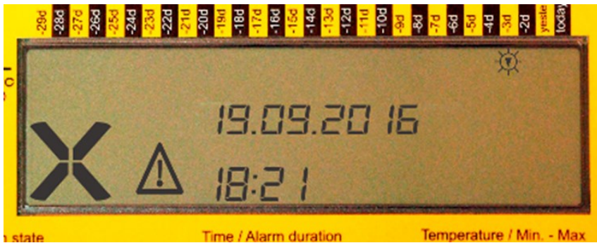
Figure 6 Visualizing the history of a Fridge-tag with preset alarm level violations – First display
