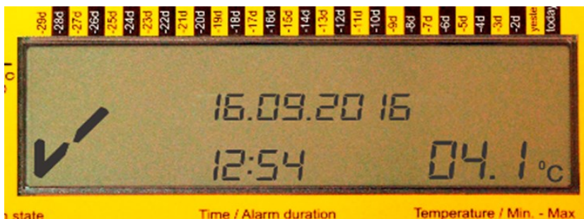
Figure 3 Current temperature reading with no preset alarm levels violation
