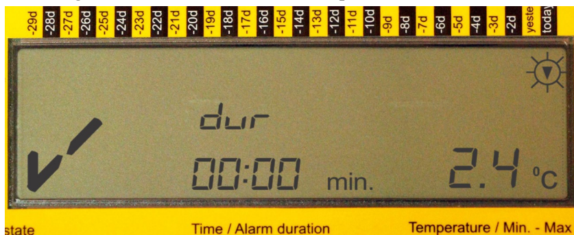
Figure 5 Fridge-tag with non-violated preset alarm levels - reading of lowest temperature
