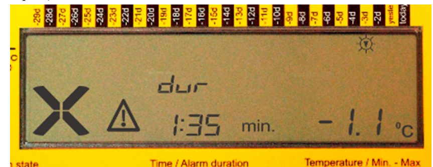
Figure 7. Display of History mode of a Fridge-tag with alarm state – 2nd display
