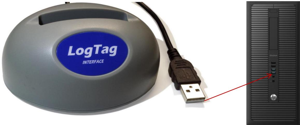
Place the logtag in the interface-when connecting, both logtag logos should face the same way.
